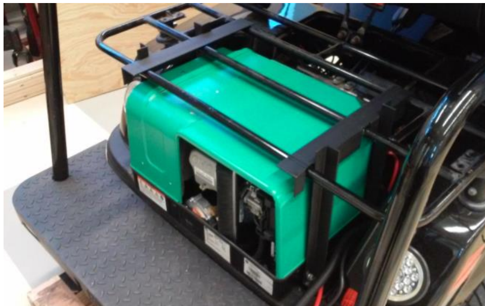
Figure 3. Photograph of the generator mount.
