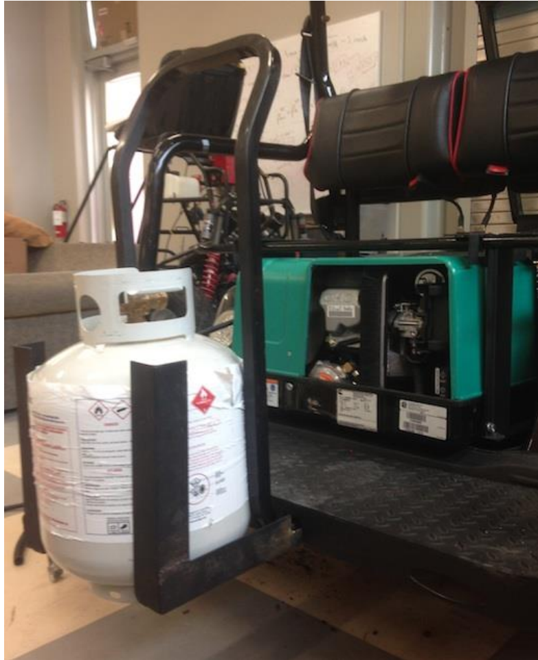
Figure 4. Photograph of the propane tank mount with the tank inserted.
